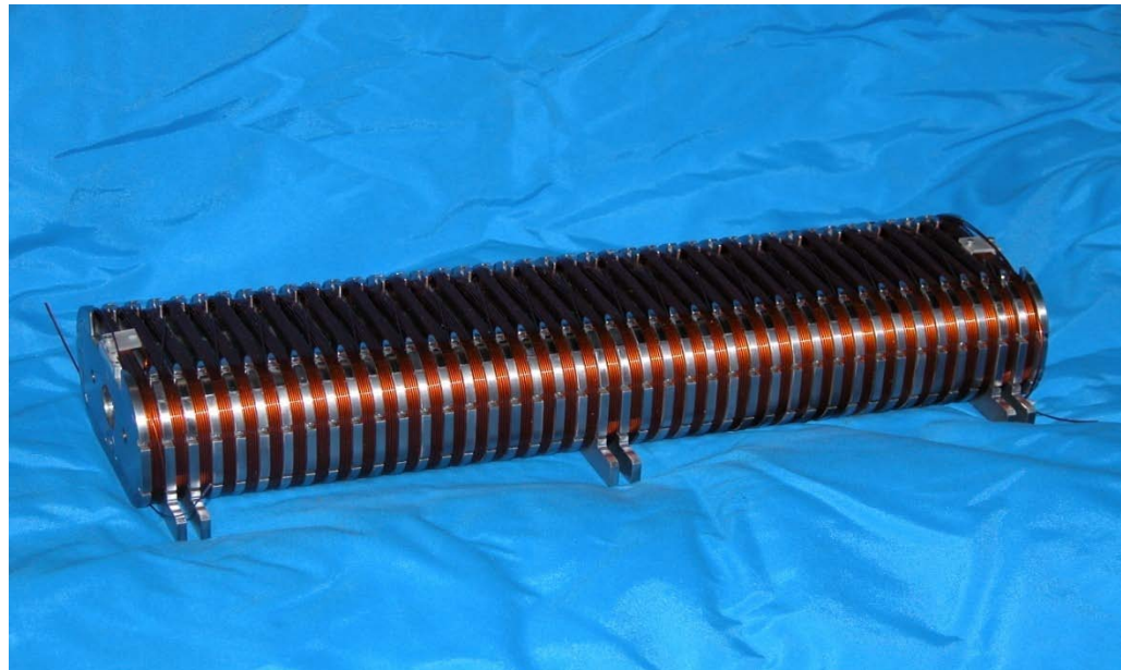
First wound 42-pole test coil
