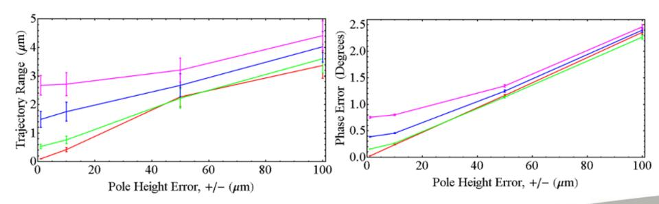
Effect of pole height error for a pole length error of ±1μm (red), ±10 μm (green), ±50 μm (blue) and ±100 μm (magenta)
