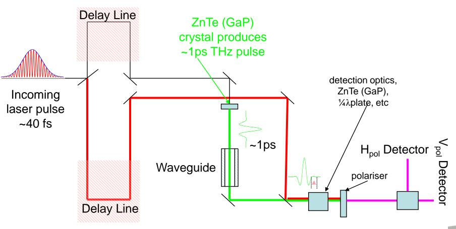
sub-picosecond time-resolved measurement of the attenuation and dispersion of a THz pulse (generated by optical rectification) through a waveguide
