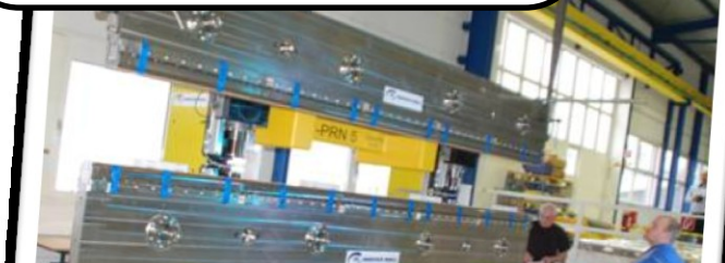
X-FEL project 5 m long undulator prototype
