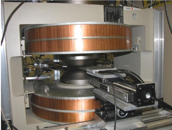
Electromagnet with a set of NMR probes
