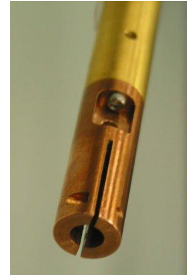
A custom-made Hall probe holder attached to a cold finger
