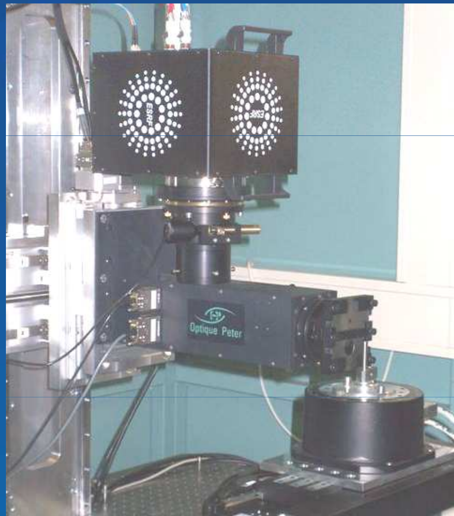
FReLoN CCD (ESRF) mounted on Optique Peter microscope (ANKA - TopoTomo-BL)
